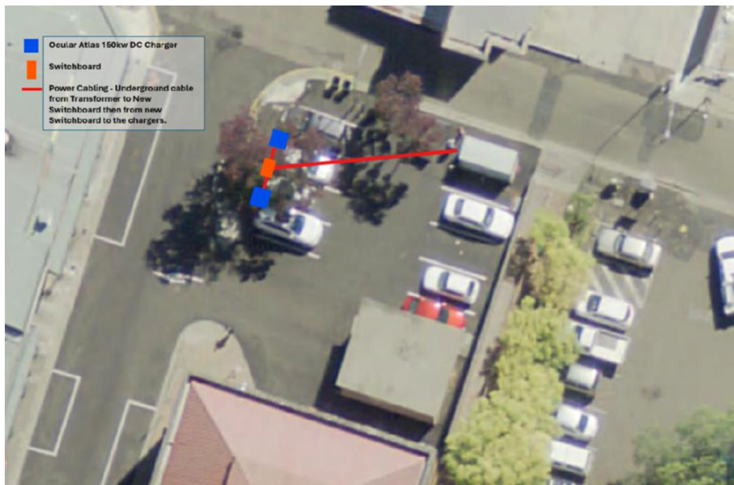
Figure 2: Indicative layout of EV charging infrastructure at 5 Cinders Lane carpark.
