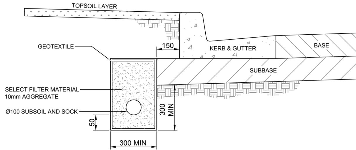
TYPICAL SECTION DETAIL OF SUBSOIL DRAIN
