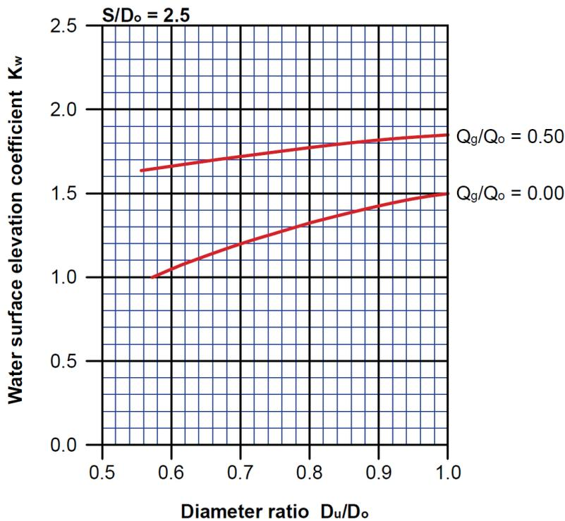
**Water surface elevation coefficients ( $K_w$ ) for  $22.5^\circ$  bends at pit junctions with branch point located on the upstream face of pit for a submergence ratio  $S/D_o = 2.5$  (Source: Hare, 1980)**
