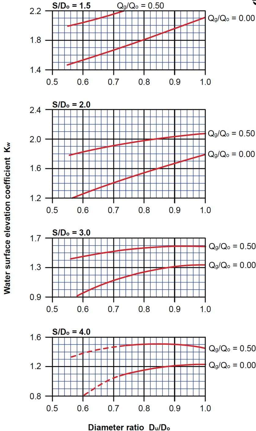
**Water surface elevation coefficients ( $K_w$ ) for 22.5° bends at pit junctions with branch point located on the upstream face of pit for submergence ratios  $S/D_o = 1.5, 2.0, 3.0$  and  $4.0$  (Source: Hare, 1980)**
