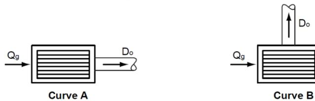
Pressure head change coefficients for rectangular inlet with grate flow only modified from DOT (1992)
