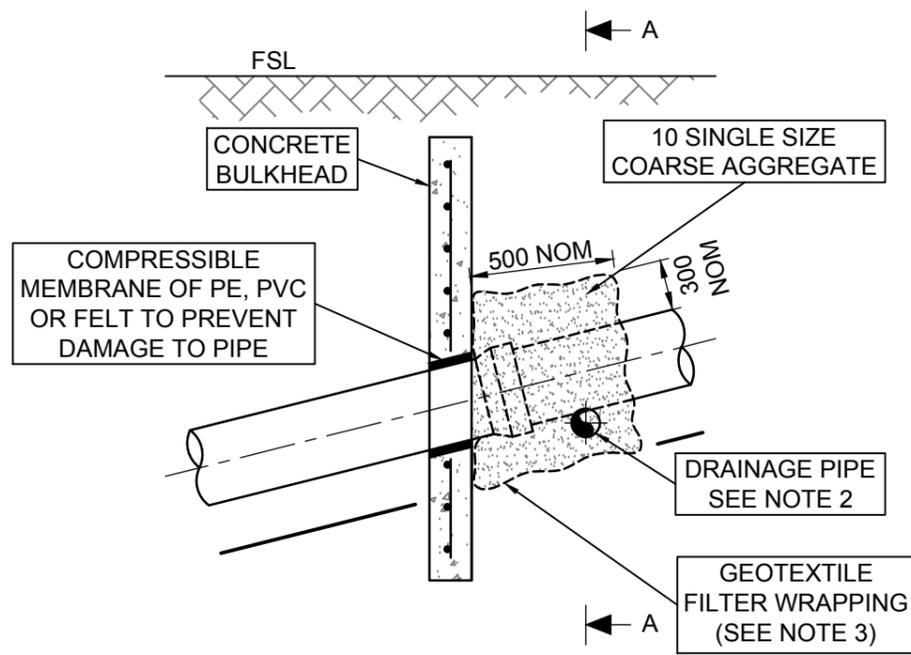
WSA FIGURE 9.18 TYPICAL TRENCH DRAINAGE DETAIL AT BULKHEAD
